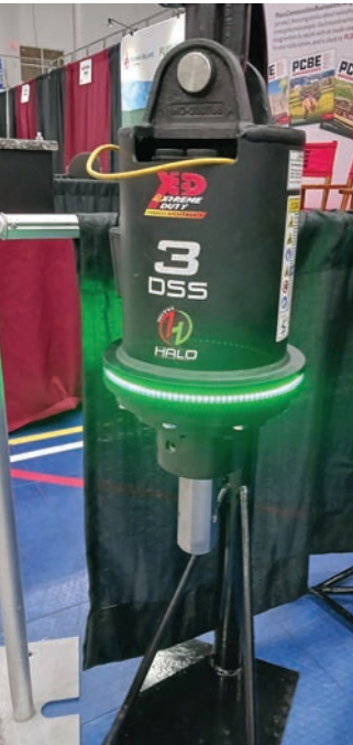
These photos show how the XED Extreme Duty auger drive indicates whether the post-hole auger is level.
