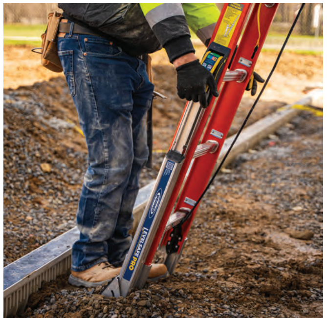
This ladder features the LevelSafe Pro ladder leveling system. PHOTO COURTESY OF WERNER LADDER.
