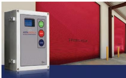
The 400HP Series High Performance Door Series features three-piece structural steel guides, minimum 3/16" steel with factory-applied UHMW anti-wear strip, and powder-coated guides, bottom bars, and headplates. It's UL325 compliant and has a springless barrel for high-cycle usage. The soft-start soft-stop DC motor reduces wear and tear, extending operational life.
