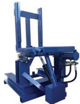
The Four Star Coil Upender is an economical solution to safely tip coils. Functioning only with a hydraulic cylinder and needle valve, it requires no electric or hydraulic hookup, making it very portable with a forklift or pallet jack. It has undergone extensive testing to ensure its safety and efficiency.
