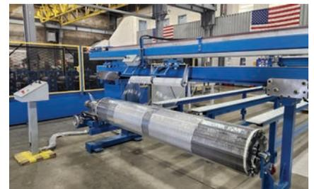
ASC's custom-designed roll-up stations allow manufacturing residential and commercial roll-up doors widths between 3.5 ft and 20 ft. Optional curtain assembly tables allow the easy pre-assembly of the door panels before the seaming process. Infeed/assembly tables feature an automated tensioning device to adjust the tension when winding seamed panels onto the drum.
