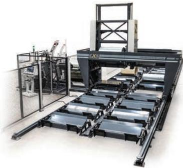
SWI's CX5 – Auto Decoiling and Storage System exceeds industry standards in reliability and serviceability as well as increased shop efficiency. The CX5 can be coupled with SWI slitters and most rollforming machines to produce automatic coil changes with a customizable range of stations and rolls up to 12,000 lbs.
