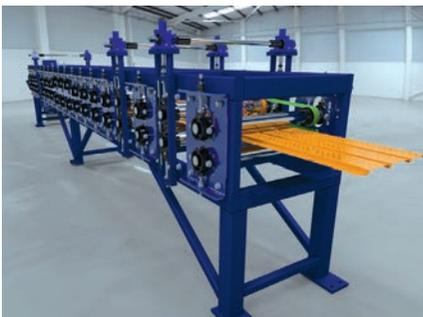
Our customer-inspired Soffit Line uses standard 20.125" coil stock to optimize inventory and cut costs. Features include concealed "S lock" lap, standard rib height, flat top rib for easy fastening, unique nail slots and weep holes for horizontal installs, and speeds over 150 feet per minute for increased productivity.
