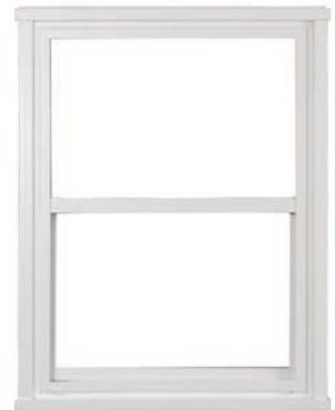
Harmony vinyl windows feature EZ-v™ trim and flashing. The exclusive EZ-V™ system permits installation into a steel-clad building with a fully trimmed panning frame that accommodates the raised ribs of the building skin. Designed for 1" nominal rib height steel, EZ-V™ reduces labor, is leak-free, paintable, and needs no J-Channel.
