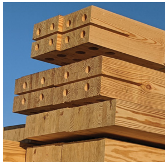
Special connection details can be utilized in glulam columns for concealed base plates. (PHOTO COURTESY OF TIMBER TECHNOLOGIES)
