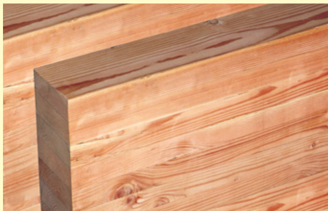
Glued laminated timber, or glulam, is engineered for a host of residential and commercial construction applications.
