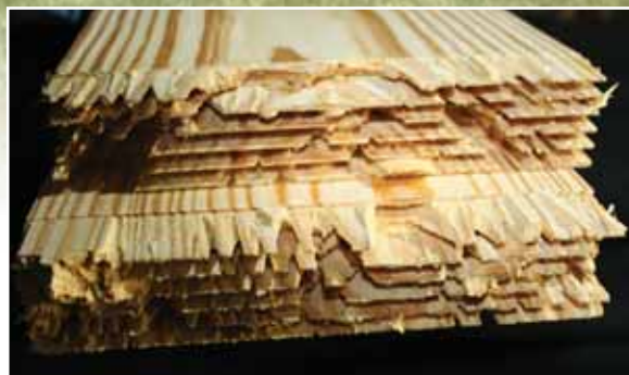
Tension Test / This particular finger joint tension test took 51,000 total lbs to break. PHOTO COURTESY OF TIMBER TECHNOLOGIES, INC.
