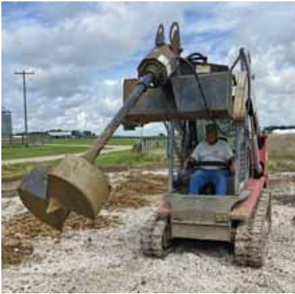
The Badger post-hole cleaner eliminates the need for a skilled worker to spend time cleaning loose soil from the post hole. Anyone who can operate a skid-steer can do the job without breaking a sweat.
