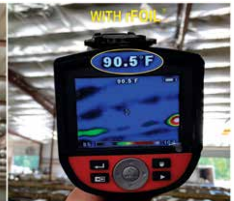
Reflective insulation can make a huge difference on the internal temperature of a building. It helps limit heat gain in storage sheds, machine sheds, ag buildings, and more. Photo courtesy of rFOIL Covertch.
