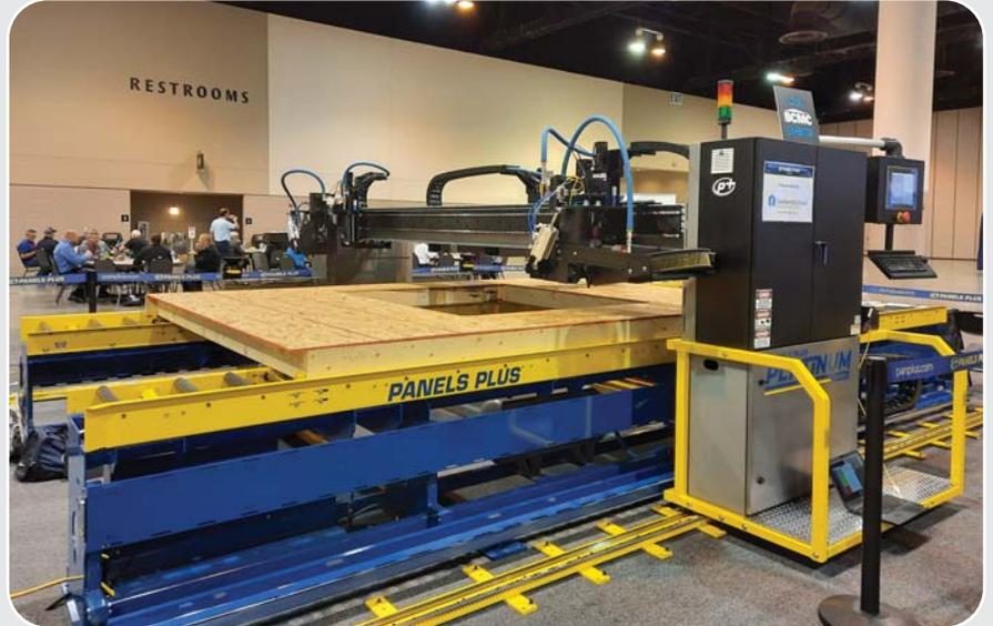
Panels Plus, an Innovance company, which uses MiTek software, debuted its Platinum Series Automated Sheathing Bridge, which offers more automation to maximize worker productivity. Sheathing stations fasten sheathing to wood wall panels made with lumber from 2x4 to 2x10. [www.panplus.com](http://www.panplus.com)
