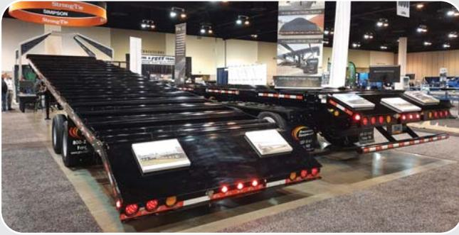
Precision Equipment Manufacturing makes truss roller trailers in standard and gooseneck configurations. The company, which marked its 20th anniversary this year, promoted its new split-roller design at BCMC 2021. The new design gives the hauler the ability to load two loads and unload at two different sites. Extension trailers are available to accommodate really long loads. [www.precisionequipmfg.com](http://www.precisionequipmfg.com)
