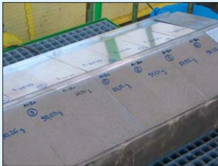
Chamber with steel samples in place.
