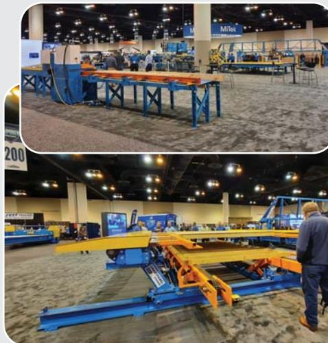
At 15,000 square feet, MiTek had the largest exhibit space at the 2021 BCMC. One of the machines on display was its prototype SmartPanel Stacker. Another machine on display was the Hornet Saw (inset), which cuts studs to length and marks stud placement, speeding construction time. [www.mitek-us.com](http://www.mitek-us.com)
