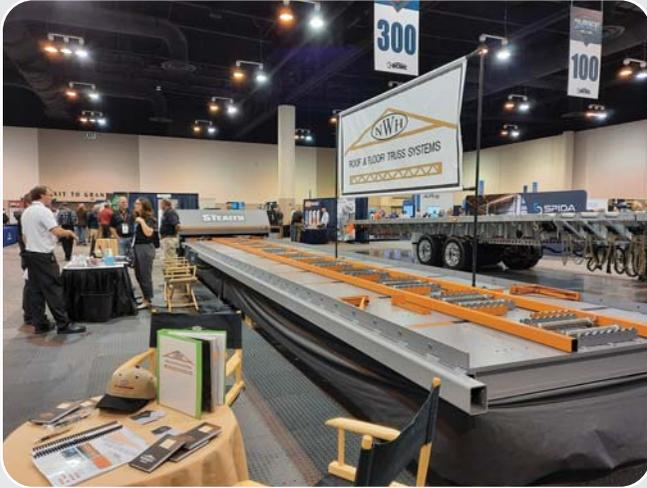
↑↑ (New Way Holdings) NWH Roof & Floor Truss Systems exhibited its Stealth Floor Truss Machine, which, with 2 workers on each side, makes quick work of cranking out floor trusses. [www.nwhtrussystems.com](http://www.nwhtrussystems.com)
