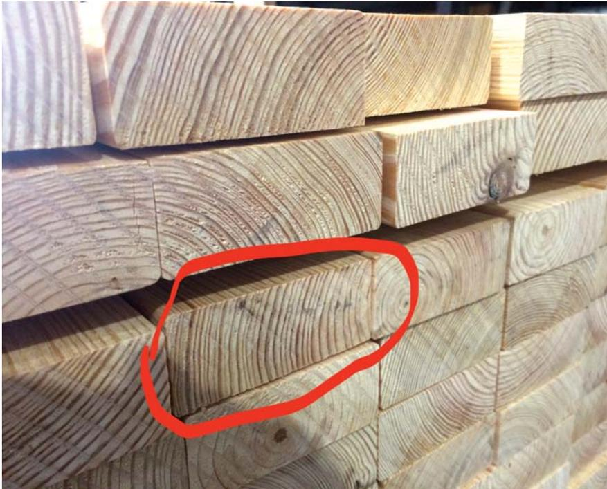
Figure 2. Best grain orientation in premium quality studs. Note the tighter growth rings in these high quality studs. PHOTO BY JACOB PRATER
