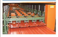
The Bradbury BOSS<sup>™</sup> Series is a stateof-the-art roll former and closed-loop servo shear with speeds up to 300 fpm and accuracy of 1/16". The BOSS<sup>™</sup> can be close coupled to a new or existing roll former. The Bradbury Group has the complete panel line solution for all production and budget requirements. Configurations include precut, post cut, Single High, Double High®, and Rafted® roll formers with flying or stop-to-cut shears.
