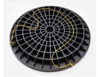
FootingPad brand isolated post footings has introduced a 20" diameter footing. With over 300,000 sold, FootingPad has reduced the labor cost in thousands of buildings. These composite footings are lightweight and easy to use, saving labor and equipment wear and tear. The new 20" FootingPad has a load capacity of over 6,500 pounds and joins a line of four other sizes, with the largest, 24", carrying loads over 9,300 pounds!
