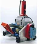
Kynar-finished Galvanize/Galvalume at 30 fpm without damage to the material. They can seam NTM, Knudson and ESE profiles! The Model SSX will form a complete double-lock standing seam with a single pass. Our exclusive nose switch cuts the unit off if it comes to the edge of the roof, eliminating expensive and timeconsuming accidents.
