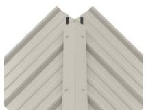
MWI's Uni-Seal® eliminates the need for angle-cut closures and is available in 20' rolls with factory-applied glue-strips: 1"x1"x20' and 1-1/2"x1-1/2"x20'. This valley and hip closure material consists of a polyurethane foam and has a vinyl coating. The continuous double glue strip is UV Stabilized and Fire Retardant.
